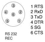
1 Connect the RS232 interface to the external printer with the AK540/ S cable.
