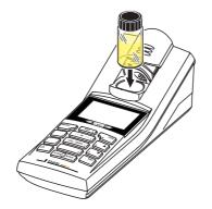
3 Align the cell marking (3) with the marking (4) of the cell shaft. The cell is ready to be measured.
